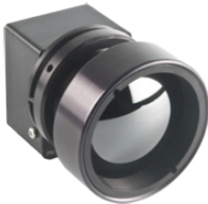
Figure 1: Tamarisk320 camera and 35mm lens. Length 49mm; weight 64g.
