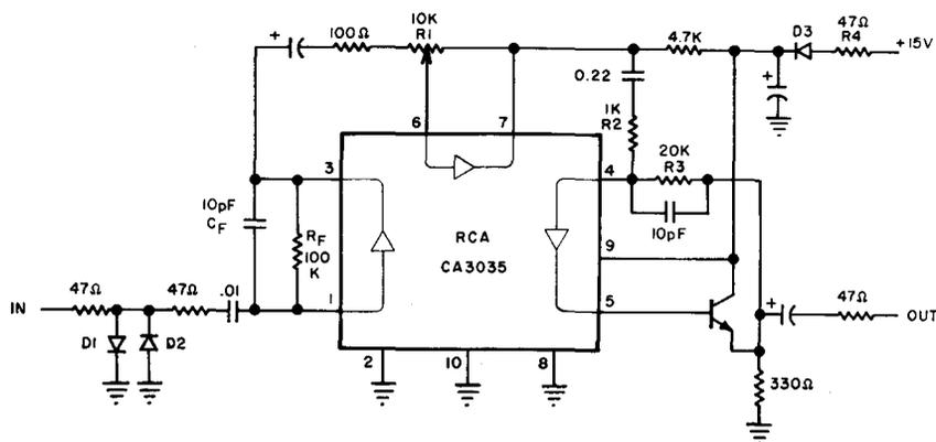
FIG. 1. Schematic diagram of the amplifier. Diodes are 1N914A or equivalent. Polarized capacitors are  $3.3 \mu\text{F}$ , 15 V tantalum. The transistor is a 2N3904 or equivalent.
