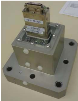
Figure 17: FEE extending from single-detector/FEE vibration fixture for component-level test
