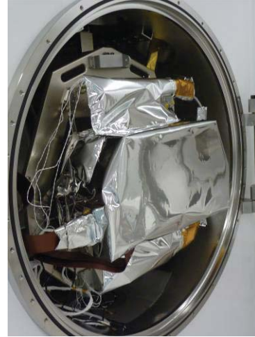
Figure 21: 4x8 demonstrator blanketed in MLI, installed in thermal vacuum chamber. Flex harnesses visible in lower left.
