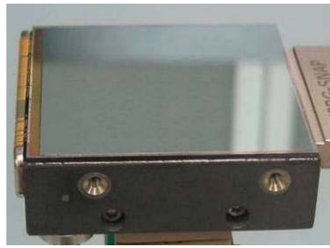
Figure 8 2k x 2k, 18 \mu\text{m} pixels, 1.7 \mu\text{m} cutoff HgCdTe NIR detector hybridized and mounted on SNAP/JDEM custom, flight configuration, 4 side abutable, SiC pedestal.
