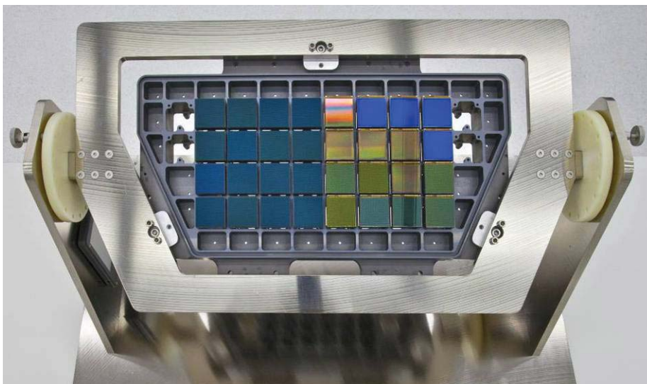
Figure 2: 4x4 array of LBNL CCDs installed to the left, 4x4 array of Teledyne H2RG ® NIR detectors located to the right. Additional detector mount positions for guiding detectors and calibration photodiodes are outboard of the 4x8 array. Detector pitch is 44.1 mm.
