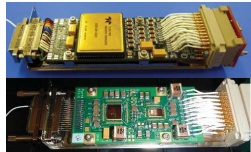
Figure 9. Top, 32-channel NIR detector readout module with TIS SIDECAR ® ASIC. The right connector mates to the detector. Bottom, CRIC-CLIC ASIC module for a CCD. The connector on the right mates to the CCD detector module.
