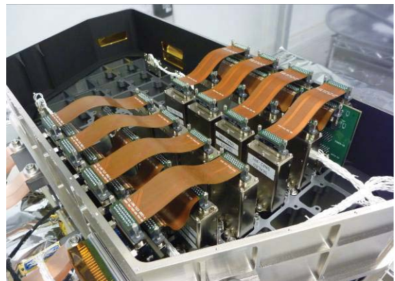
Figure 5: View inside the half-populated rear enclosure, showing FEEs, flex circuits, and quadrant boards
