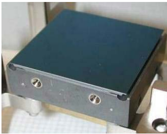
Figure 7. Back-illuminated SNAP/JDEM CCD mounted on flight configuration 4 side abutable SiC pedestal. The format is 3.5k x 3.5k, 10.5 \mu\text{m} pixels with four corner readout. The CCD is 200 \mu\text{m} thick for extended red response.
