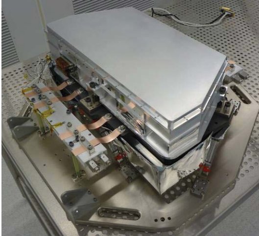
Figure 20: 4x8 demonstrator being prepared for thermal vacuum testing. Cold finger and thermal straps visible to the left.
