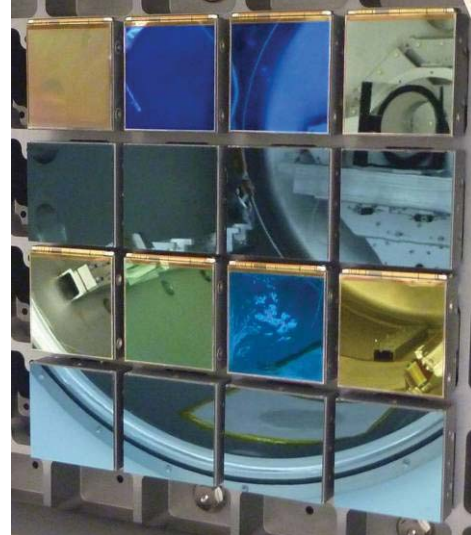
Figure 12: Photo of two quadrants populated on the focal plane. CCDs and NIR detector rows alternate, with NIR on the top row, followed by CCD row, and so on. The detectors in the third row down are NIR detectors and were susceptible to parallel clock interference from the CCDs just above them, while the top row of NIR were not. Note that the NIR wire bonds and flex circuit are adjacent to a row of CCDs. This was the likely area where noise was coupling into the H2RG ® outputs, and was easily shielded.
