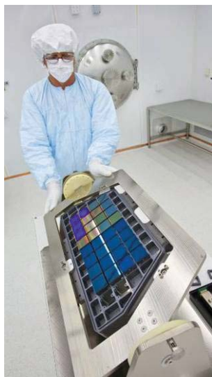
Figure 1: 4x8 Cold Plate in handling fixture, with 16 CCDs and 16 NIR detectors
