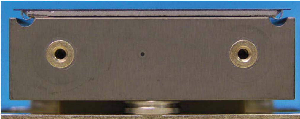
Figure 14: End view of complete packaged CCD. Two threaded inserts seen here are two of the three available for a detector guard or filter frame. Precision spacer visible at bottom in middle. The wirebonds can be seen in the two troughs.
