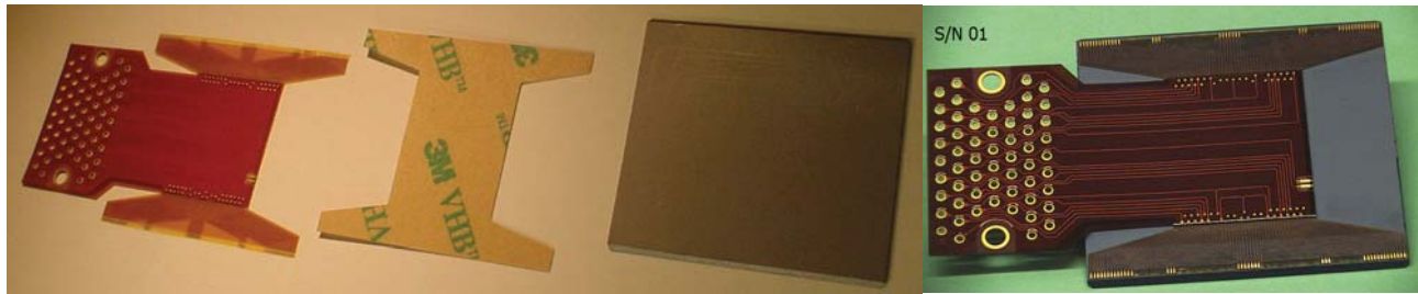
Figure 3: Flex circuit, PSA, and substrate separately (left) and assembled (right)
