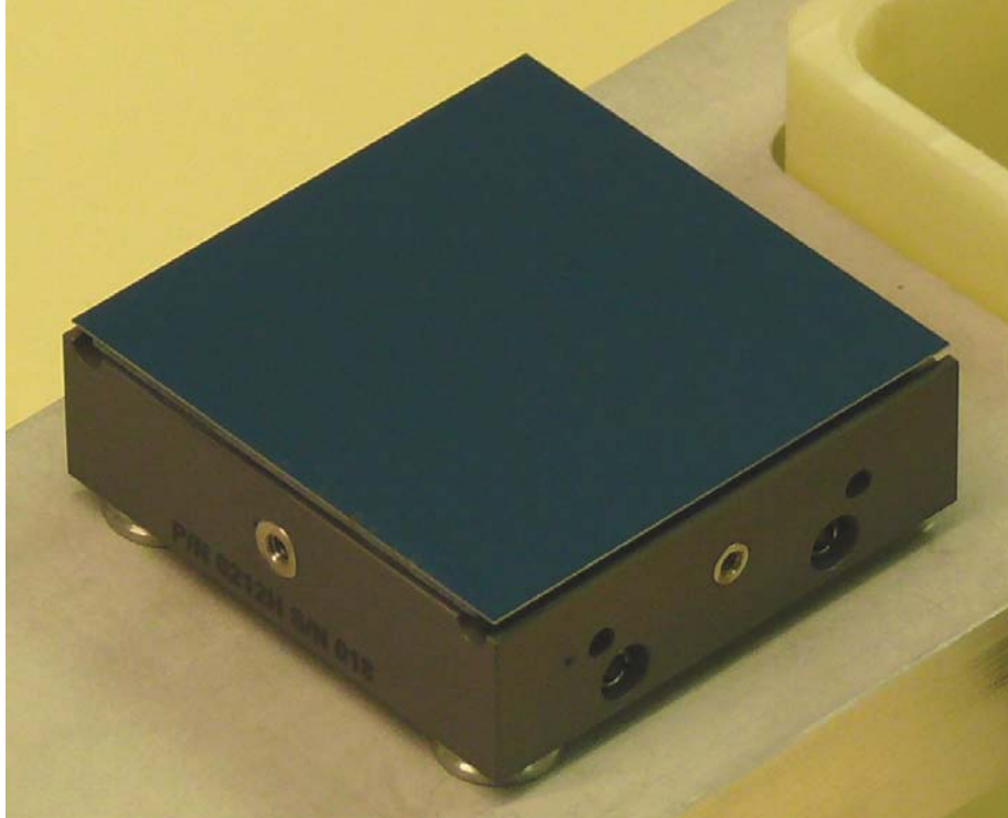
Figure 13: Complete packaged CCD on precision spacers. Threaded insert on the left is one of three available for mounting a detector guard or filter frame. The insert to the right is for handling.
