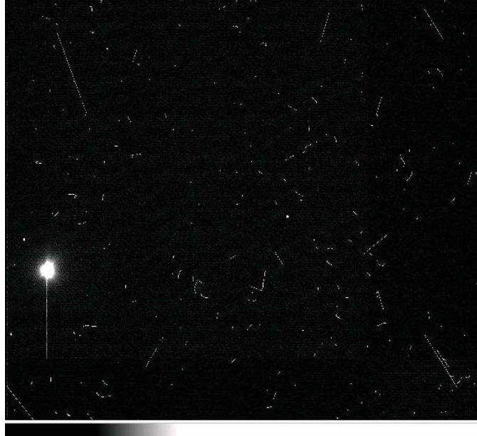
Figure 11. An 1800 second dark exposure of the completed package showing cosmic ray and lab natural background radiation tracks.
