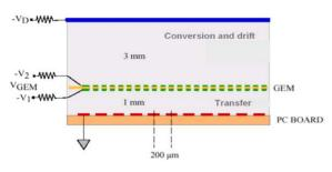
Fig. 1. View of a MicroPattern detector with pixel read-out.
