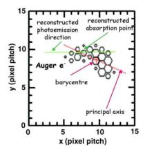
Fig. 2. Real photoelectron track. Reconstruction of the photoemission direction is done with the identification of the absorption point and the removal of the final part of the track, where directional information is lost due to track randomization Coulomb scattering.
