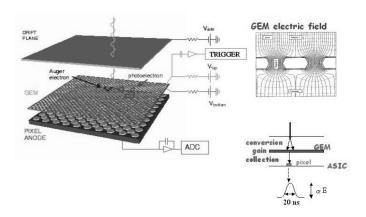
Figure 1. The Concept of Micropattern Gas Chamber
