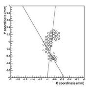
Figure 2. The track produced in the gas by a 5.9 keV photon is recorded by the MPGC and analyzed with the following sequence: barycenter evaluation; reconstruction of the principal axis; reconstruction of the conversion point; reconstruction of emission direction. The polarization is derived from the reconstructed angular distribution of the photoelectrons.
