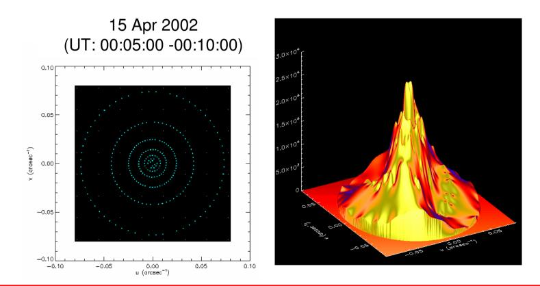
The idea is to use the FFT2D algorithm on the smoothed visibility surface produced by the interpolation algorithm
