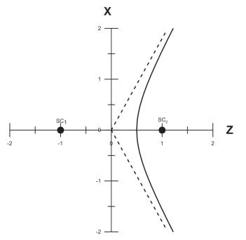
**Figure 1.** Two-dimensional example of GRB triangulation when the source distance is allowed to vary. The two spacecraft, 1 and 2, are aligned along the *z*-axis, and are the foci of a hyperbola. The hyperbola defines the loci of the possible source distances. If the distance is assumed to be infinite, the two possible GRB arrival directions are along the asymptotes (dashed lines).
