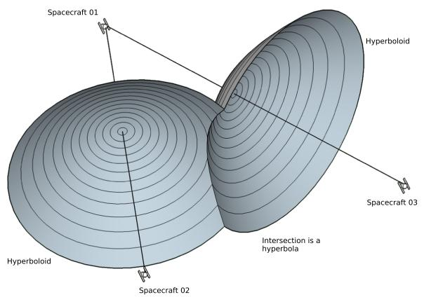
Figure 3. Intersection of two hyperboloids. With detections from three spacecraft, each spacecraft pair constrains the location of the source to a surface of a hyperboloid. The intersection of the two hyperboloids is a simple hyperbola contained in a plane. The point on this hyperbola that is closest to Earth gives the lower limit to the source distance.
