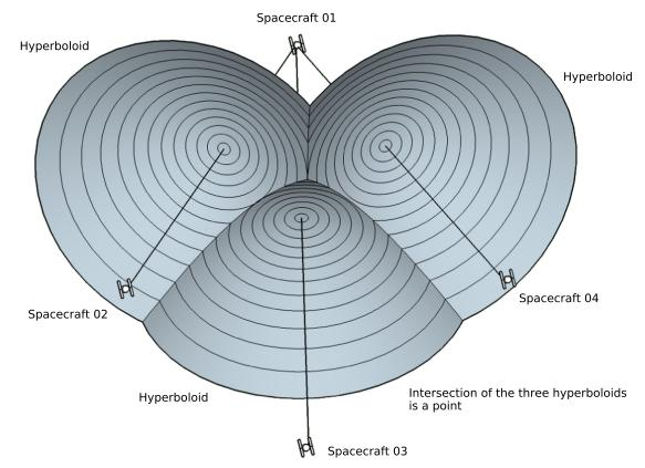
Figure 4. Intersection of three hyperboloids. Using detections with four widely separated spacecraft, each spacecraft pair constrains the location of the source to a surface of a hyperboloid. The intersection of the three hyperboloids is a point in space as illustrated in the figure. In this case, one can determine the source distance purely by timing measurements.
